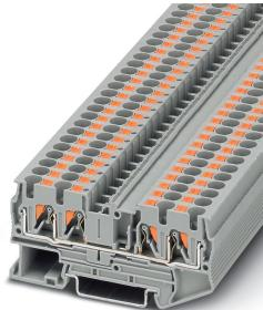
Feed-through terminal block, nom. voltage: 800 V, nominal current: 32 A, connection method: Push-in connection, 1 level, Rated cross section: 4 mm<sup>2</sup>, cross section: 0.2 mm<sup>2</sup> - 6 mm<sup>2</sup>, mounting type: NS 35/7,5, NS 35/15, color: gray
