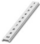
Zack Marker strip, flat, Strip, white, labeled, Printed vertically: consecutive numbers 1 ... 10, 11 ... 20, etc. up to 91 ... 100, mounting type: snap into flat marker groove, for terminal block width: 6.2 mm, lettering field size: 5.15 x 6.15 mm, Number of individual labels: 10
