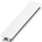
Zack marker strip, Strip, white, unlabeled, can be labeled with: PLOTMARK, CMS-P1-PLOTTER, mounting type: snap in, for terminal block width: 6.2 mm, lettering field size: 6.15 x 10.5 mm, Number of individual labels: 10
