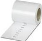
Marker for terminal blocks, Roll, white, unlabeled, can be labeled with: THERMOMARK ROLL 2.0, THERMOMARK ROLL, THERMOMARK ROLL X1, THERMOMARK ROLLMMASTER 300/600, THERMOMARK X1.2, THERMOMARK S1.1, perforated, mounting type: snap in, snap into flat marker groove, for terminal block width: 6.2 mm, lettering field size: 6.35 x 6.15 mm, Number of individual labels: 16000
