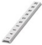
Zack Marker strip, flat, Strip, white, labeled, printed horizontally: consecutive even numbers 2 ... 20, 22 ... 40, etc. up to 82 ... 100, mounting type: snap into flat marker groove, for terminal block width: 6.2 mm, lettering field size: 5.15 x 6.15 mm, Number of individual labels: 10
